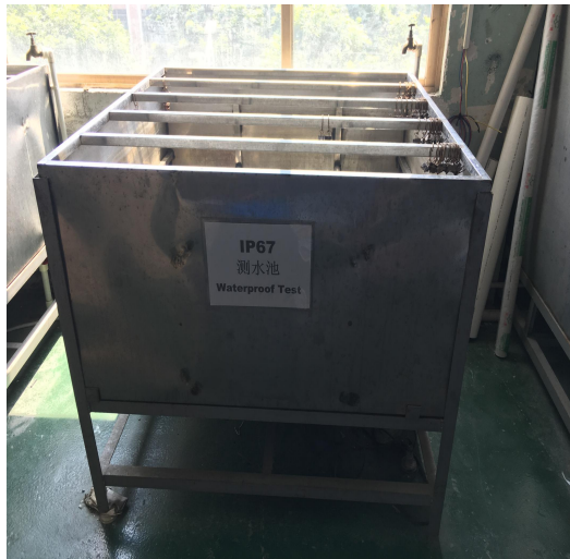
Water tank for IP66/67 test
